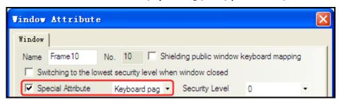
**2** Right-click the mouse in the blank area in the Frame10 window to select [Group]-[Use the group element], then select [keyboard] from [Group Components] in [Edit Box of Group Components Library], and select the right keyboard from [Preview] and click [Place Group Components] button, then the keyboard will appear in Frame10.
