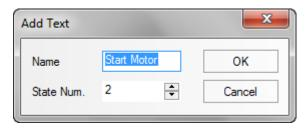
For example, build a text item named "Start Motor", the State Num is 2, each text supports 256 states at most. Click on the Ok to finish building the text, and click on the Cancel to give up this text.
