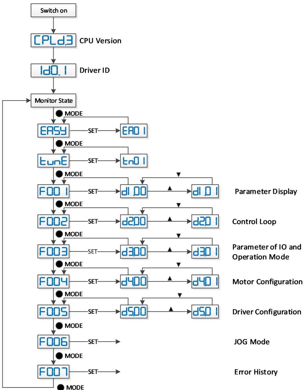
Figure 4-1: Parameters setting
