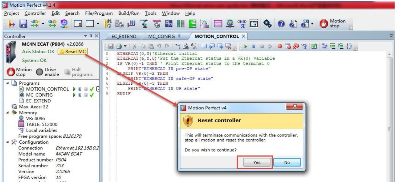
After successful reset, the frame like below (it needs 2min at least for this controller when reset and power on). At the middle area, it is project information file. At left side, it shows the status of controller and slave driver. At right side, it shows the information in window channel 0 that the Ethercat initial program has been executed successfully and the system has found Kinco FD slave which is in Ethercat OP state (Operation state) also.
