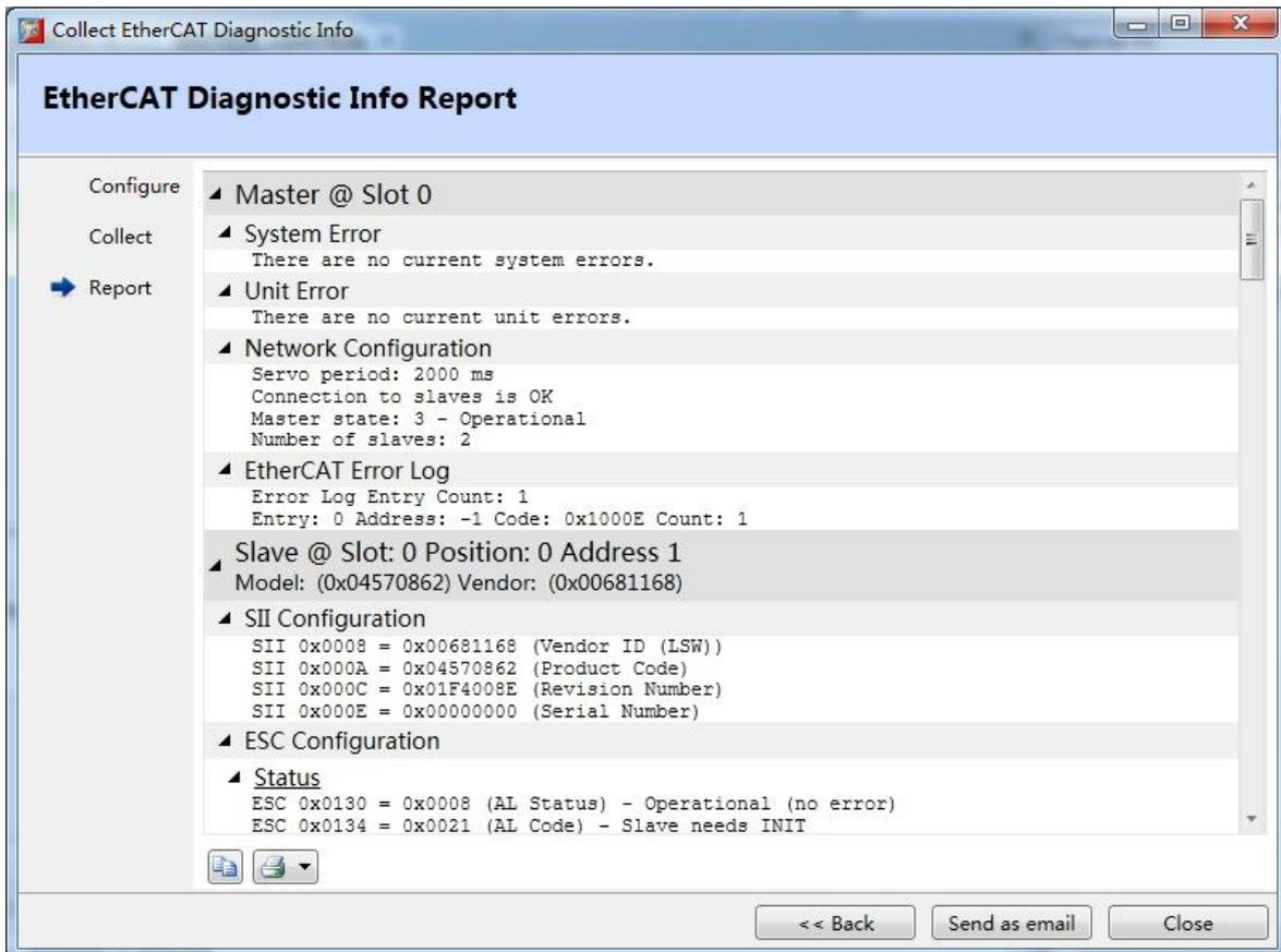
At the same time, it can be found in Kincoservo software that the master has configured PDO to driver and connected with driver successfully. In others table, it shows that if there is sync data or not. If non-zero value is changing continuously, it means there is sync data and is updating also. Meanwhile, if the statue LED of Ethercat on driver is on constantly, it means under operation state.
