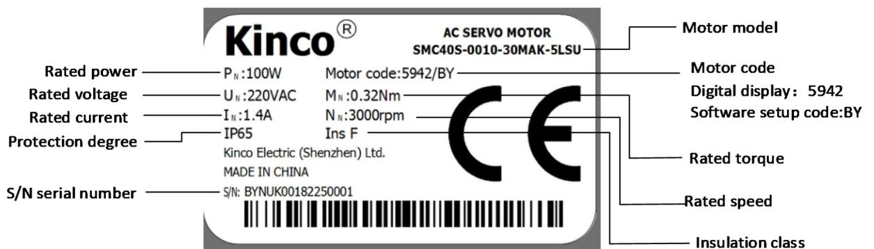
Figure 1-4 Motor nameplate description
