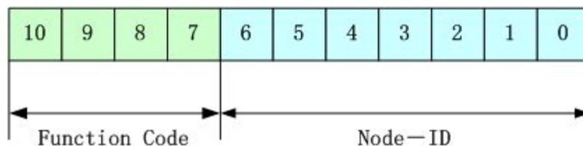
Node-ID is defined by system integrator, such setting by the DIP switch on the devices (Like servo's station
