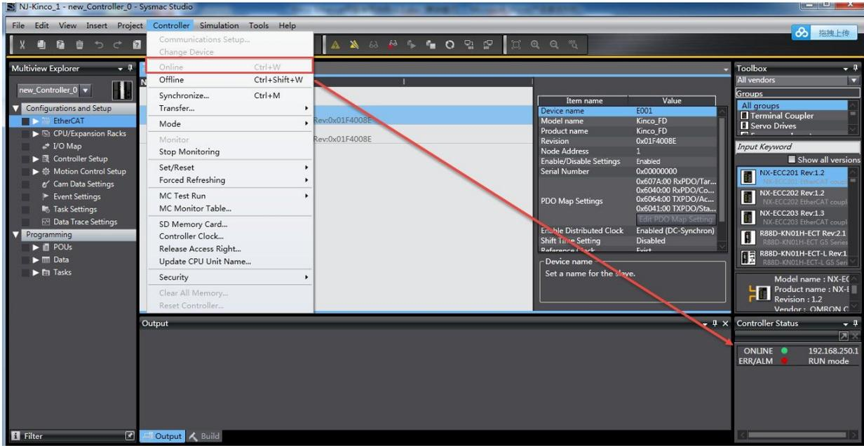
Controller-Synchronize. After synchronization, it will show what the different is by comparing with program and parameters of controller inside and local program in PC. Click Transfer To Controller and click Yes into program mode and then click Yes into run mode.
