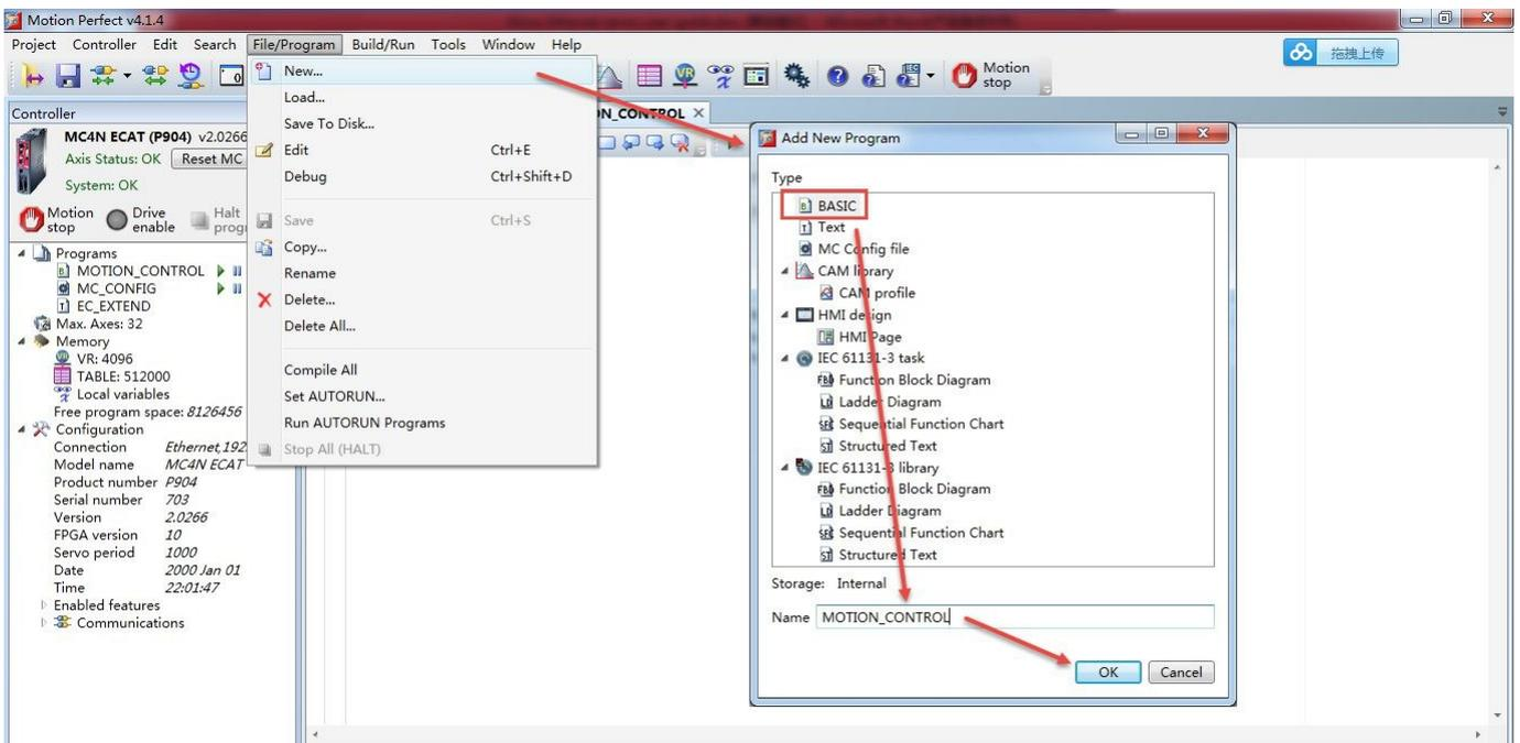
Write a Ethercat initial program then save and compile. Finally, open a terminal window on channel 0 to display related information.
