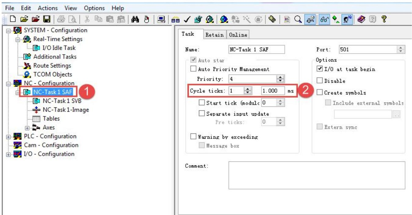
Click Enable for Sync Clock, should be noted that the setting of Cycle Time here must be same with ECAN sync cycle(the value in 301101 also) in driver. For example if the sync cycle is 2(4ms) then here should be 4. It will make the servo vibrated when running if the cycle is different.
