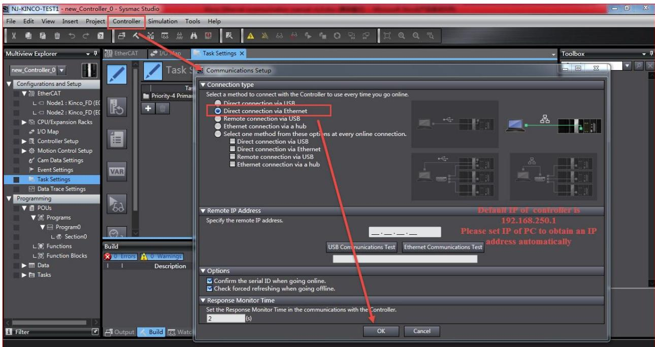
Open software Direct Ethernet Utility and choose Direction connect target.
