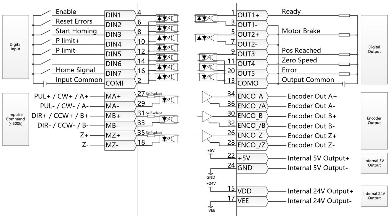
Figure 4-4: X4 wiring in pulse train mode
