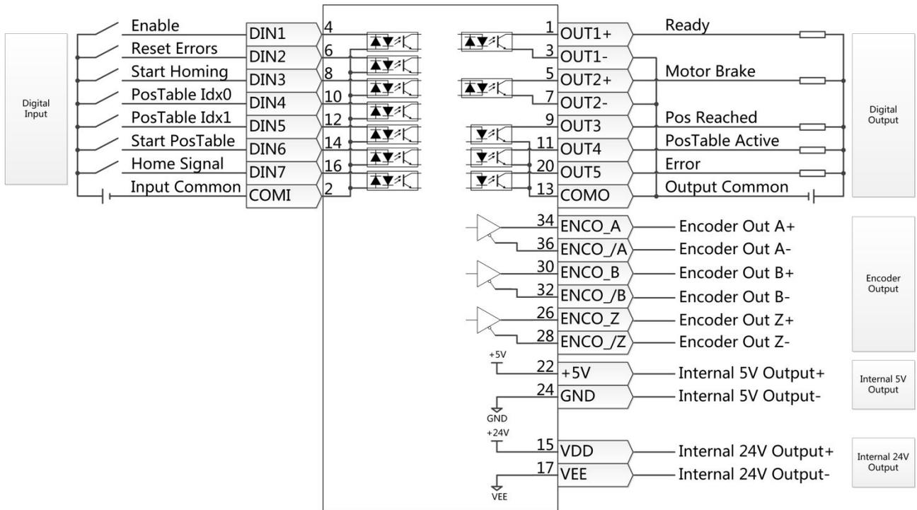
Figure 4-6: X4 wiring in position table mode
