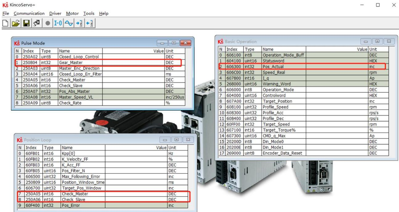
Figure 6-9 Full-closed loop master-slave axis inspection Settings
