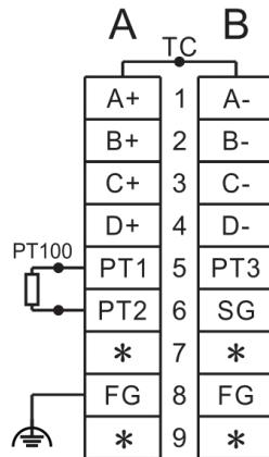
Fig.8.3.4-1 2-wire PT100 cold junction external compensation wiring
