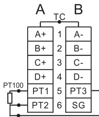
Fig.8.3.4-2 3-wire PT100 cold junction external compensation wiring
