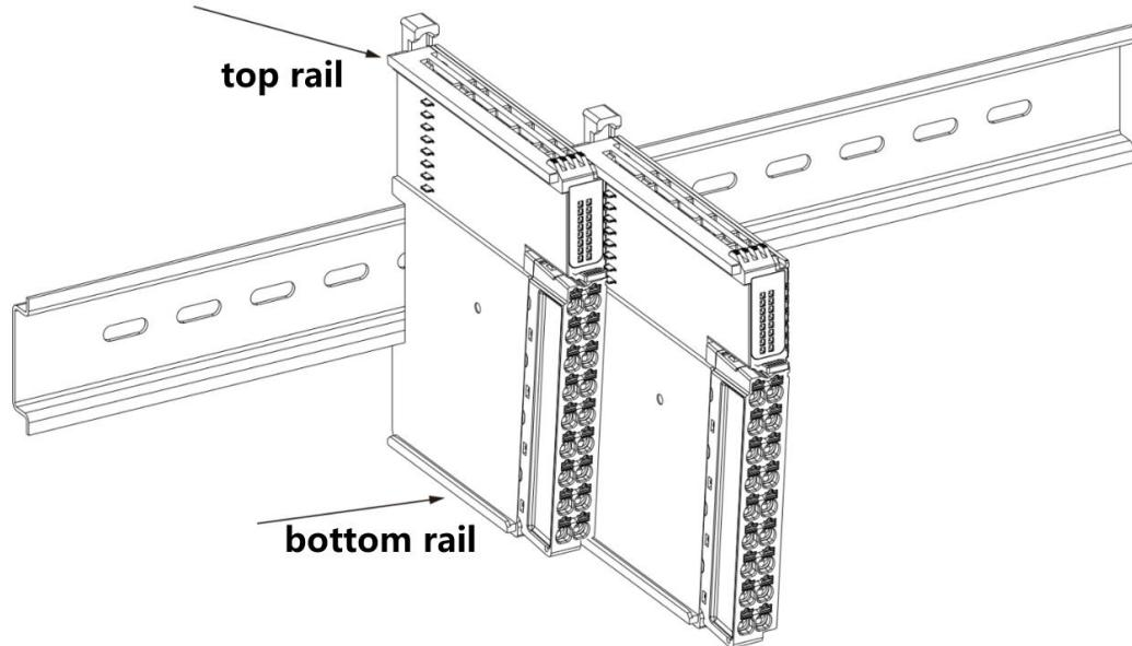
Fig.10.2-2 Module assembly
