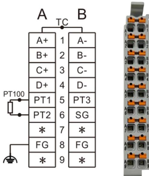
Fig.7.3-1 RP20-0400TC wiring diagram
