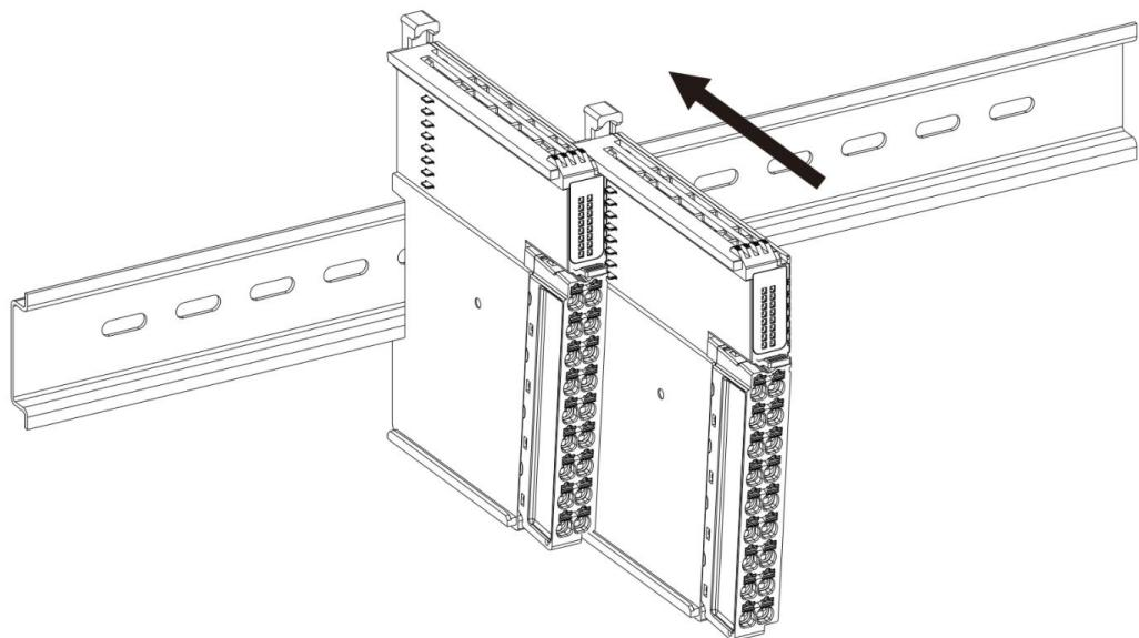
Fig.10.2-3 Module assembly
