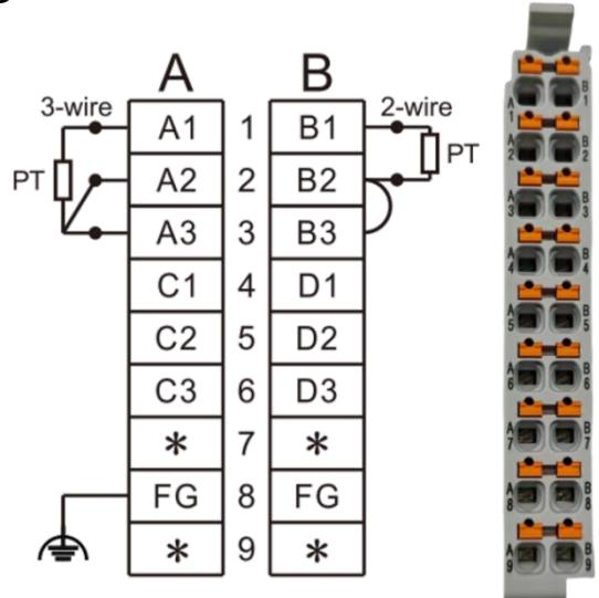
Fig.7.2-1 RP20-0400RD wiring diagram
