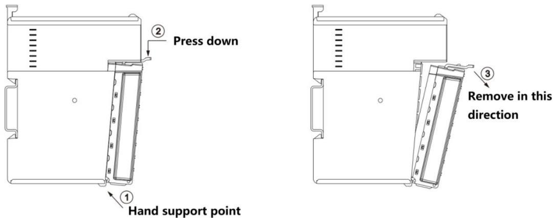
Fig.10.2-7 Connector disassembly
