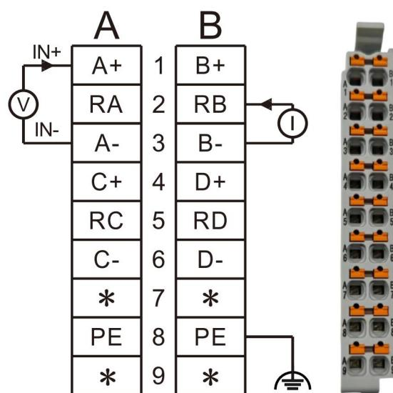
Fig.7.4-1 RP20-0400IV wiring diagram
