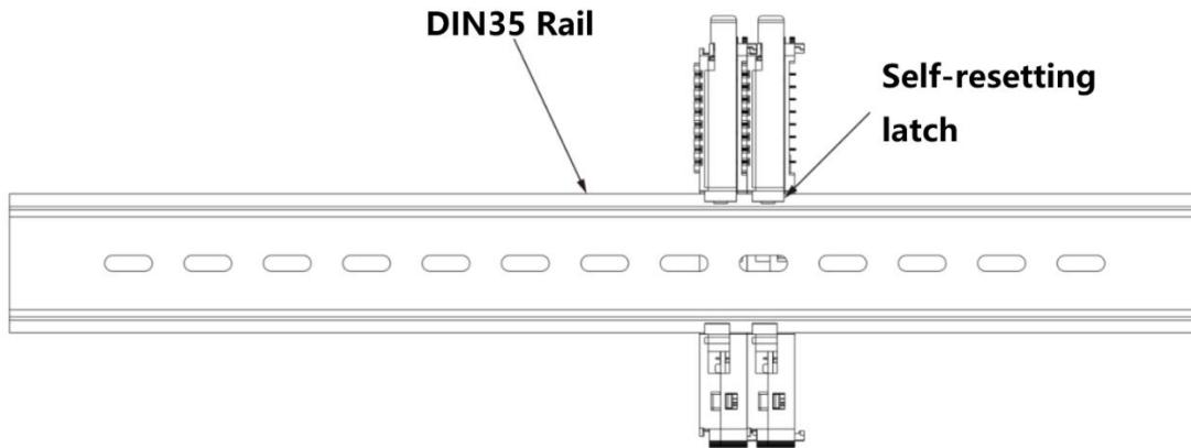
Fig.10.2-4 Secure the module onto the DIN35 rail
