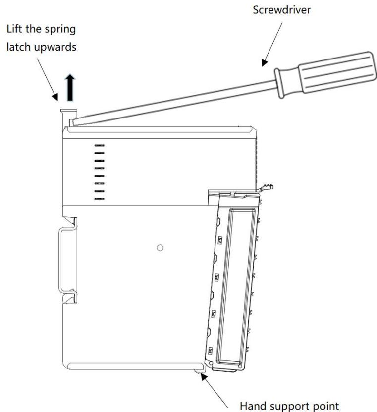
Fig.10.2-6 Module disassembly
