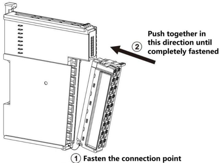
Fig.10.2-8 connector assembly
