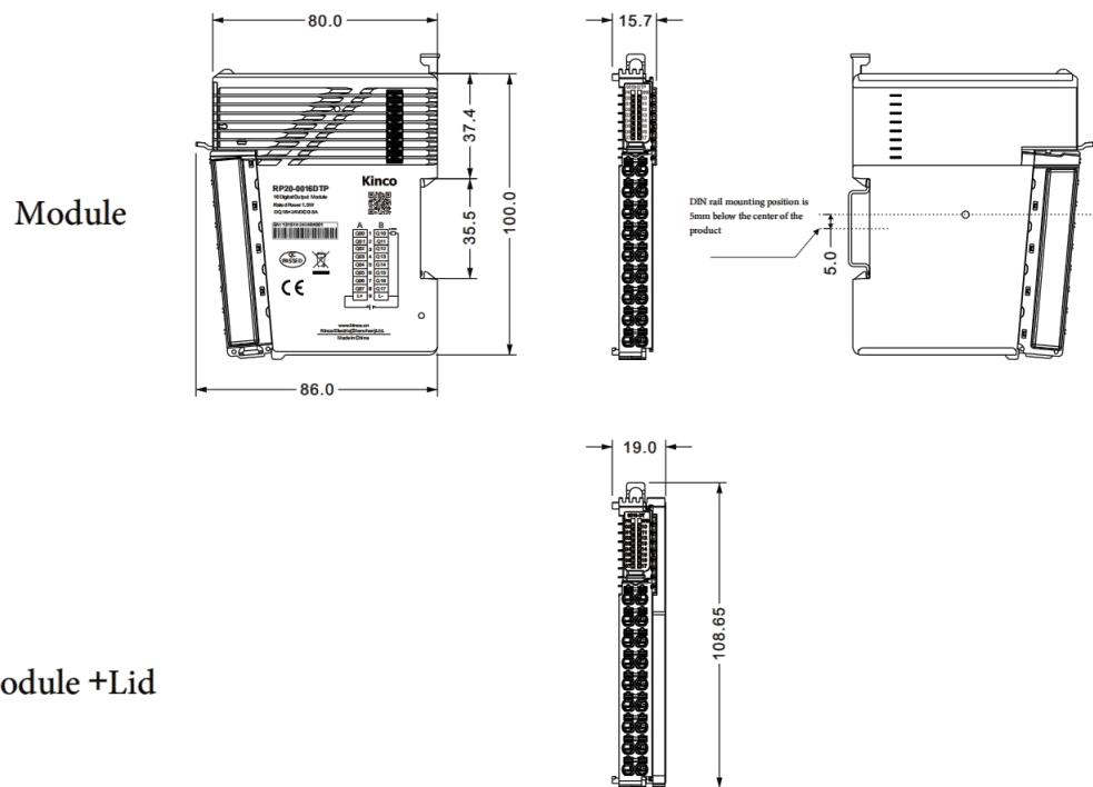
Fig.10.1-1 Installation dimension
