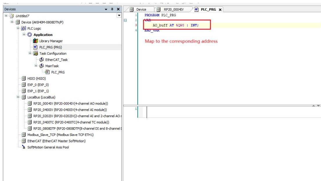
Fig. 11.2.2-4 Map the desired address to a custom variable
